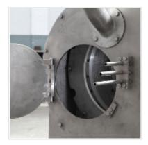
Our pusher centrifuge is the continuous filtering type centrifuge used for solid-liquid separation in industries of chemical, light industry, fertilizer, salt and food, etc.
