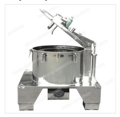
The PBZ vertical top discharge centrifuges are equipped with direct shaft connected motor. This series of filtration centrifuge features base plate, manual discharge and batch-type operation. Customers avail from simple structure, reliable performance and ease of operation. Adjustable filtration time is responsible for efficient washing and undamaged solid phase.
