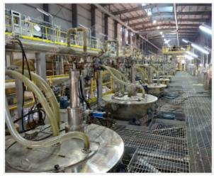
The SGZ three-column automatic bottom discharge scraper centrifuges are mainly applicable for washing of slurries containing solid phase as well as solid-liquid separation. The suitable solid phase size is 0.05-1mm, and filtration cake density is limited from 1.0 to 1.5. The solid content in slurry is ranged from 15% to 50%. Moreover, slurries should be uniform and continuous, and have exceptional mobility in pipeline.
